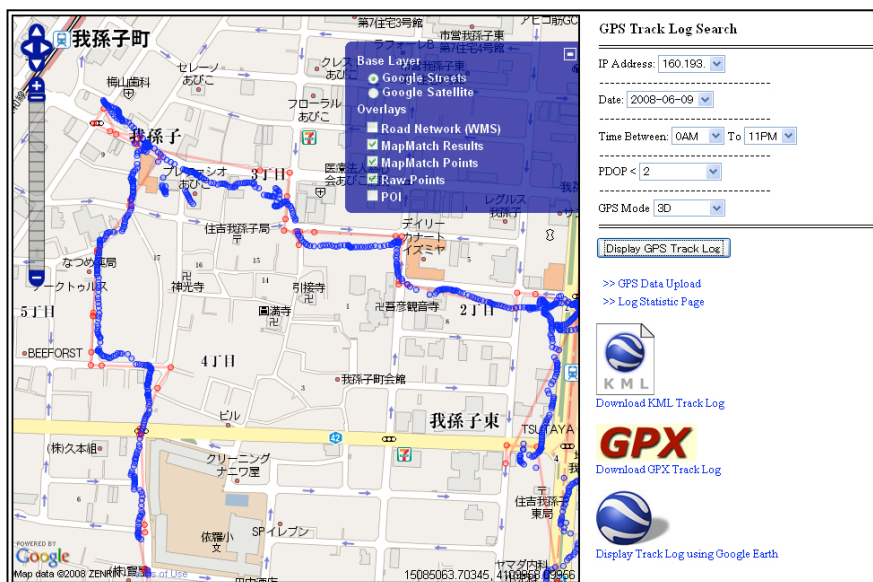
Figure 5. Track Log Search Interface using OpenLayers
